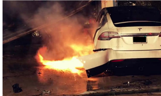
Flame jet from Tesla Model X. NBC LA, 2017.
